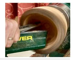
Design the piece as required but consider leaving a wider rim to show off the bark – the natural edge – & undercut to reduce the thickness of the bowl.
