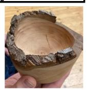
As you will read later on, the bark can come loose & fly off a turning piece. Please ensure you are using adequate PPE to protect your face & eyes when turning a natural edge. Also consider standing to the side of the firing line.
